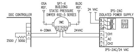
Often when powering a Dwyer 4 wire pressure transmitter, a 24VAC isolated AC supply is required to avoid ground loops with different pieces of equipment. The IPS-2AC provides two isolated 24VAC outputs rated for loads up to 250mA AC
