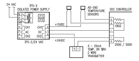
The IPS-2 isolated DC power supply is used to maintain the input isolation from the 24VAC line and provide 4 selectable voltage ranges to power various temperature sensors and 4-20mA transmitters.
