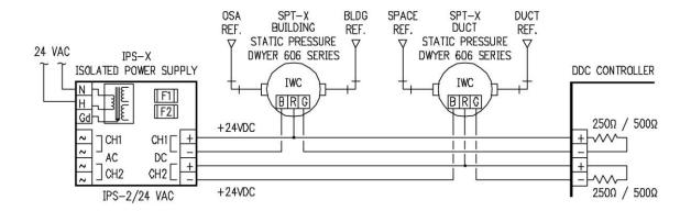
When using Dwyer's 606 3 wire 4-20mA transmitter, a separate 24VDC supply is needed for each transmitter. This is because the 606 is a positive referenced device, with +24VDC supply connecting to controller signal input and 606 red wire. The 24VDC supply common connects to 606 black wire, and the 606 signal common (green wire) connects to input common with a 250V load resistor connected between signal input and signal common.
