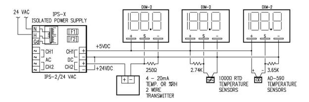
It is often required to provide multiple panel indication meters for various signal ranges. The IPS-2 has 4 selectable voltage ranges and a fine adjust trimmer per output channel to power multiple DIM-2 indicators and other DC devices.
