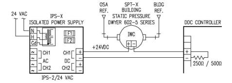
Often a 24VDC supply is required to power a number of 4-20mA transmitters such as the Dwyer 600 series. The IPS-2 eliminates the need for a separate 24VAC transformer and can provide 24VDC @ 250mA to power up to 8 current loop transmitters simultaneously.
