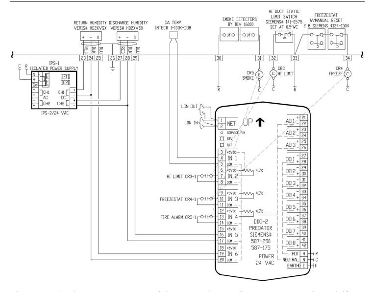
When using Veris humidity 3 wire 4-20mA transmitters & the Siemens Predator controller, a separate 24VDC supply is needed for each transmitter. This is because the input commons on the controller are not common to each other and thus one signal can effect to other.
